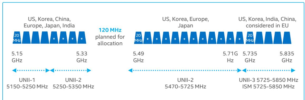
In addition to the basic frequency limits, the use of the 5 GHz bands for LTE are dictated by regulatory stipulations. Another main requirement for access to these frequencies is to ensure fair coexistence with other users in the band by implementing widely accepted technical mechanisms such as Clear Channel Assessment (CCA) and Listen before Talk (LBT).
