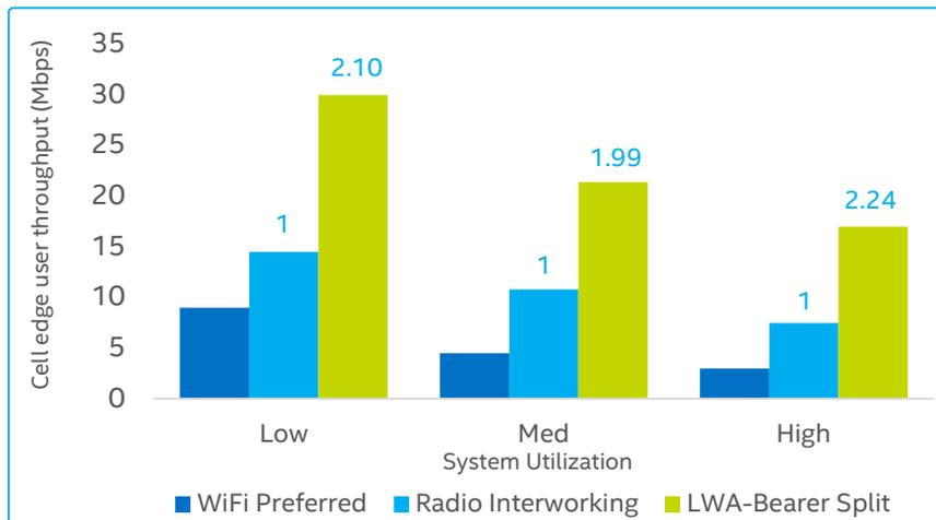
LWA's MUS algorithm outperforms the radio interworking solution with an average gain of 30% and cell edge gain of 85% across all users.
