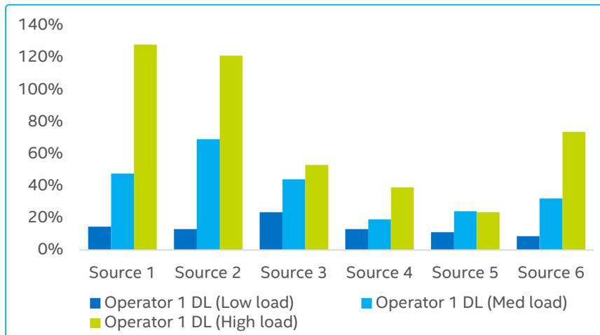
Improvement in the UPT for the DL only Wi-Fi network (Sources 1-7 are from 3GPP contributions R1-150694, R1-152732, R1-151821, R1-152863, R1-153384, R1-153426, and R1-153629, respectively.)
