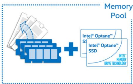
Intel® Memory Drive Technology can revolutionize your data center memory architecture. When combined with Intel® Optane™ SSDs, Intel® Memory Drive Technology transparently integrates the drive into the memory subsystem and makes it appear like DRAM to the operating system and applications. This can increase memory capacity beyond DRAM limitations, with no change required to the OS or applications.
