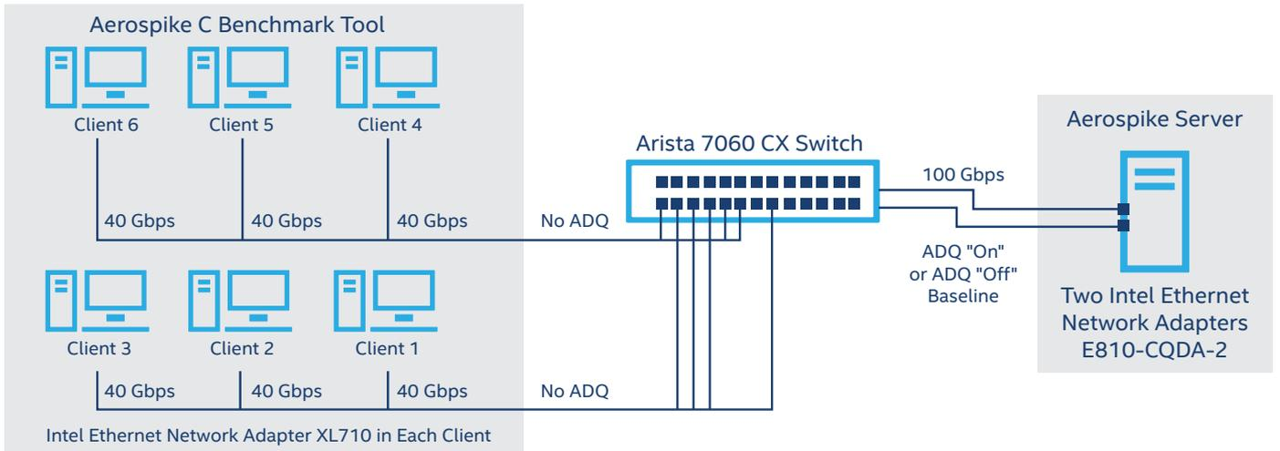
Figure 5. Aerospike test setup
