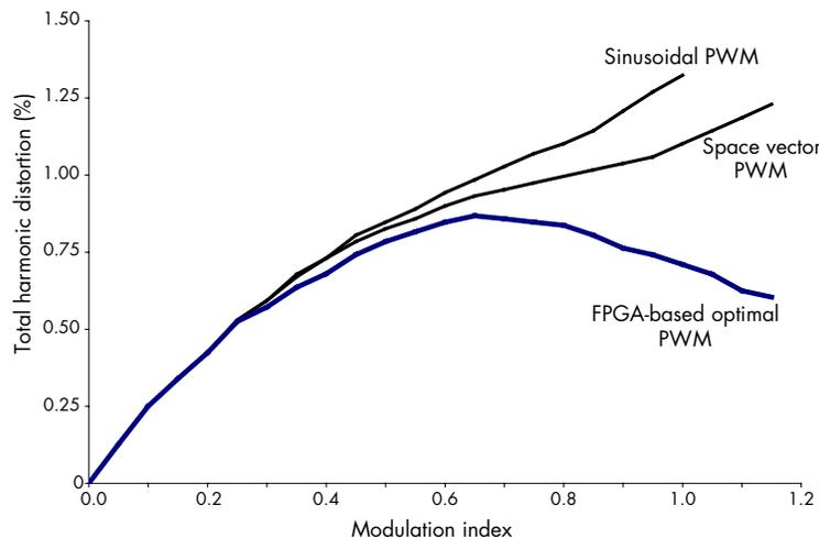
Experimental validations on PMSM show that such THD reductions may provide a 50 to 55 percent reduction of motor and power converter losses, thereby providing tremendous gains in global efficiency. These new margins of loss reduction can make the difference in helping home appliances meet Energy Star ratings and/or for designers to add new product differentiating features, such as an enhanced HDTV-based human-machine interface.
