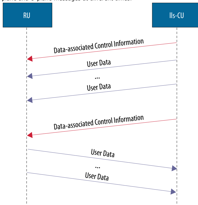
Figure 7. Scheduling control and user data transfer procedure
