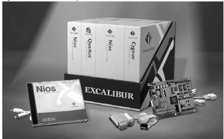
Figure 1. Excalibur Development Kit, with the Nios Embedded Processor
