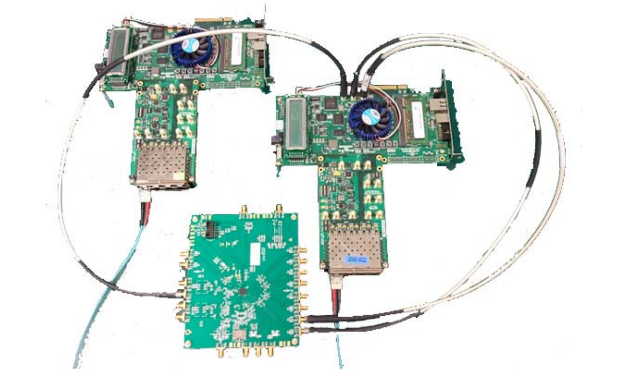
Figure 2. Dual Board Reference Design: LC Master to RRU Slave
