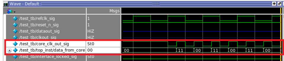
Figure 12. Interface Locked Signals from Altera PHYLite Instances
