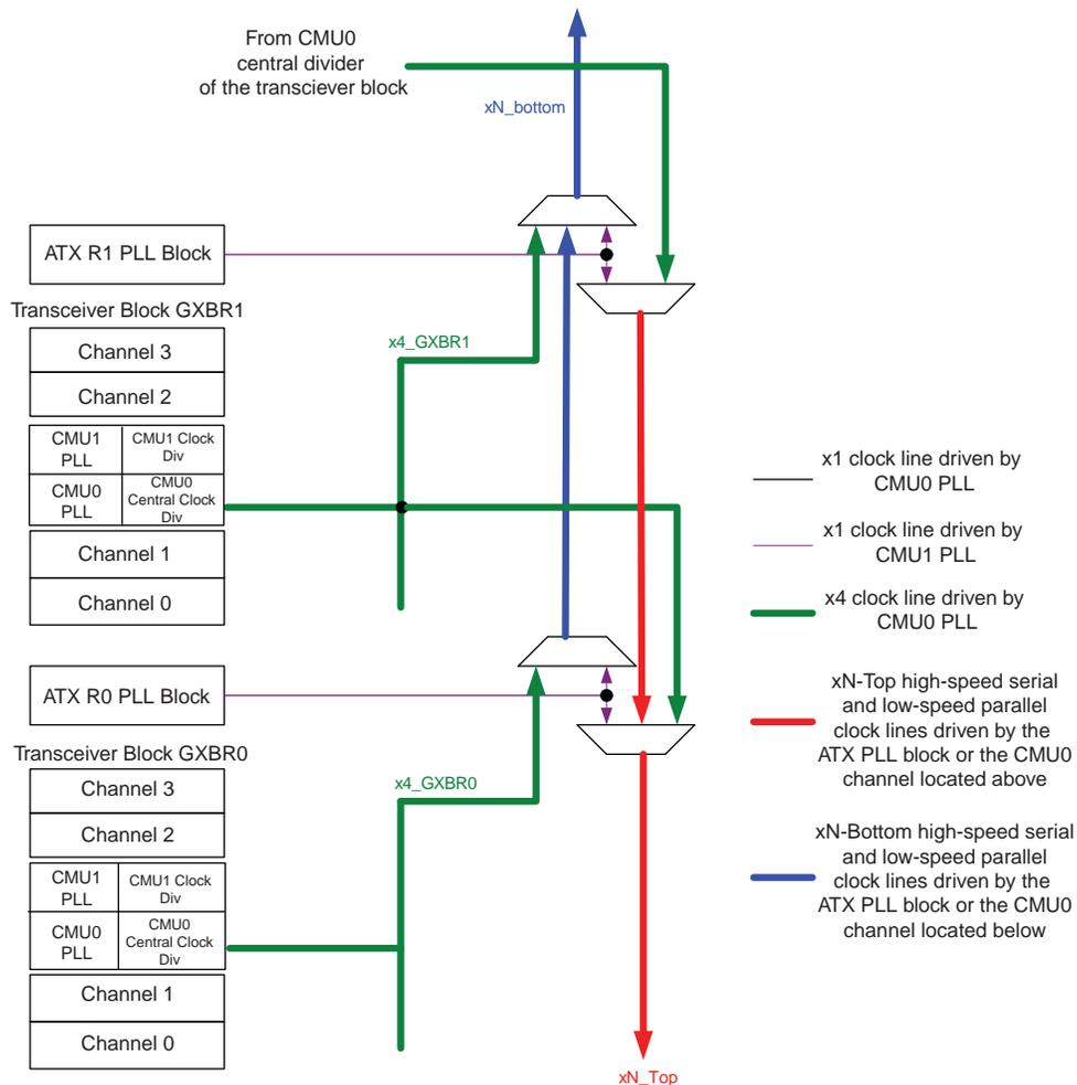
As shown in [Figure 1](#), a transceiver block in the center gets the highest number of transmitter PLLs—two CMU PLLs within the same transceiver block—one from above and one from below the transceiver block (refer to [Figure 2](#)).
