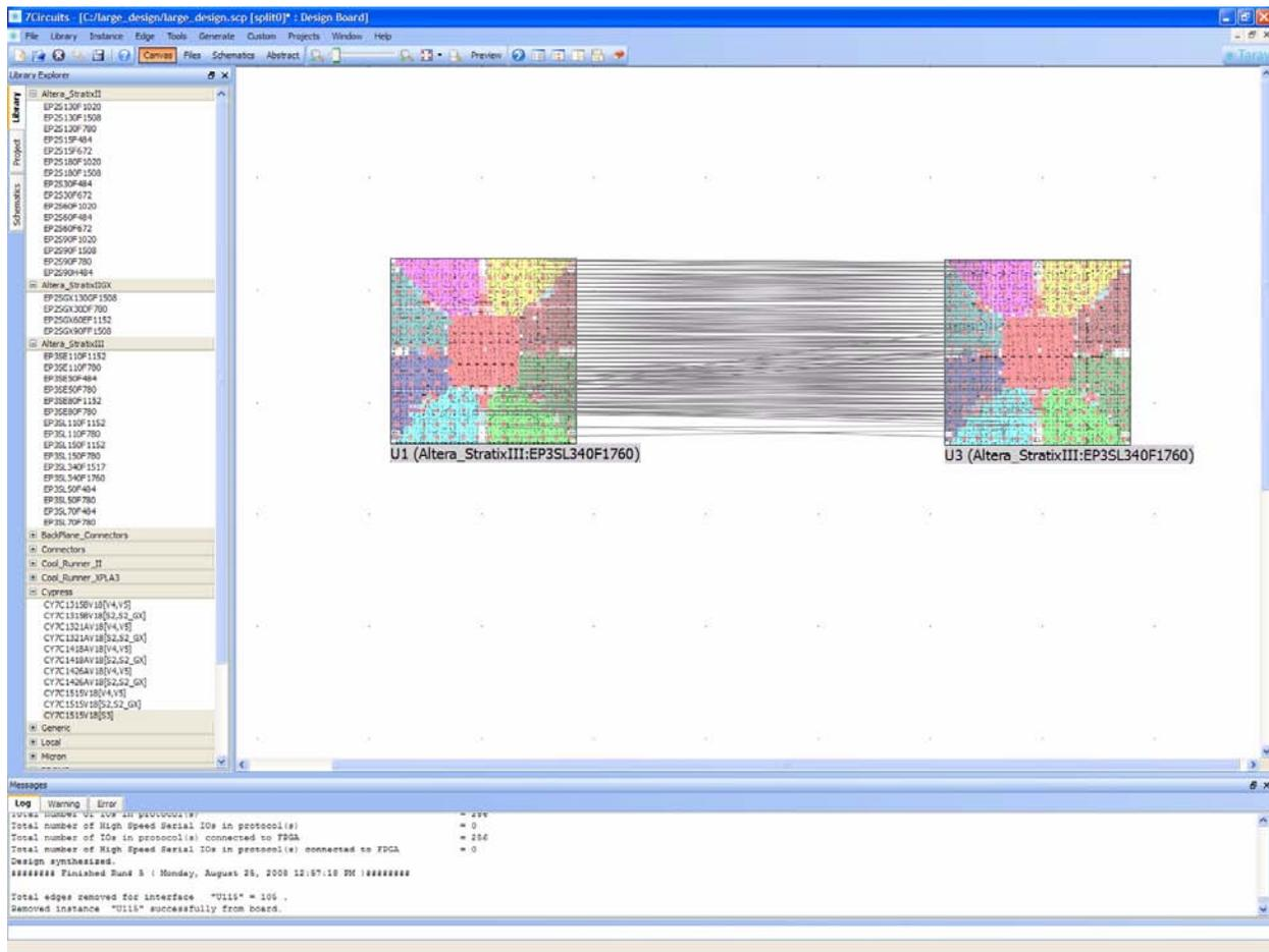
8. Edit the split as a stand-alone design. In Figure 5, a Cypress memory device has been added to the split and the design resynthesized. While not readily apparent in this figure, in order to get the Cypress device to connect to the left edge of the left FPGA (U1), the connections between the two FPGAs also had to be optimized. This is one of the benefits of working on the design at a smaller level; details like these are more obvious and easier to manage.
