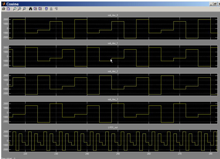
When random input data with 3.185 MHz bandwidth are used, you can set up the system as in Figure 3. In this case, the polyphase modem modulates the 3.185 MHz input signal onto 160 MHz carriers, well exceeding the device clock rate of 100 MHz. The output signal spectrum follows Figure 7.
