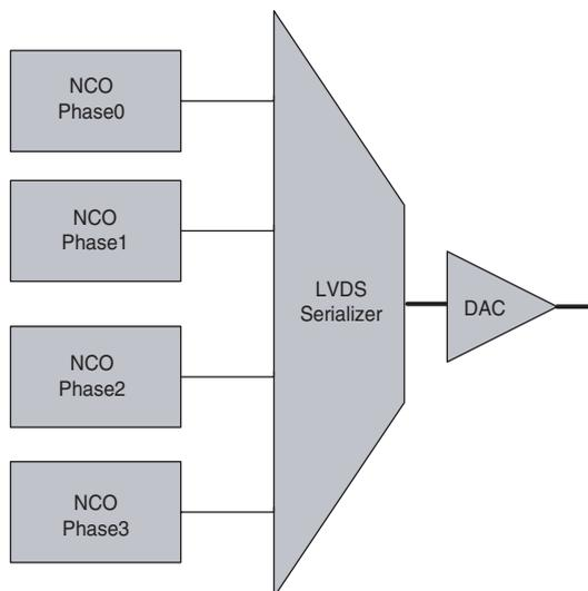
If the clock rate of the NCO is  $f_{NCO}$ , the sampling rate of the LVDS serializer is  $Nf_{NCO}$ , which equals the sampling rate of the high-speed DAC  $f_{dac}$ . Denote  $f_{out}$  as the output signal carrier frequency (in Hz) of the LVDS serializer. Define the normalized digital frequency  $\theta$  as:
