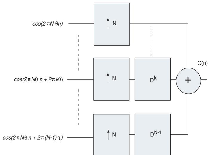
The multiplex operation of the LVDS serializer in Figure 4 can be modeled as a delayed sum of N-upsampled data sources. Therefore, the final output data off the FPGA to DAC is upsampled by an additional factor of N.  $D^k$  denotes k-sample delay. Because delay is easily modeled in the Z-transform domain, you will express the signals in the Z-domain. Recall that the Z-transform of a cosine signal is given by [3]
