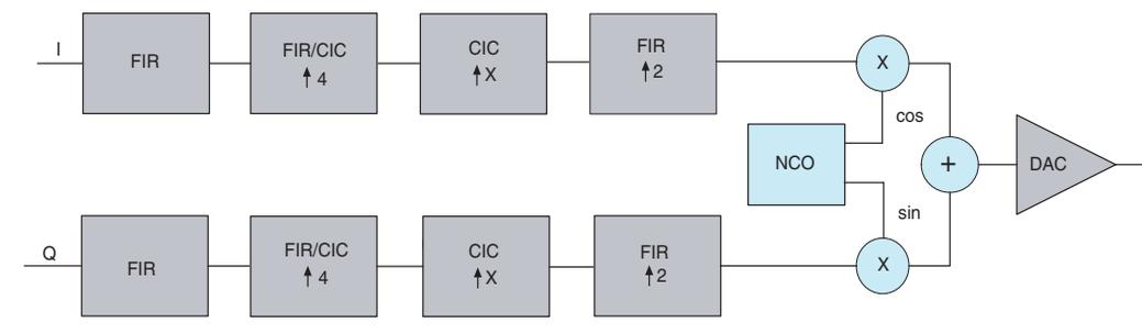
A variable rate, cascaded integrator-comb (CIC) filter can further provide a large range of rate change. It is often accompanied by a compensating finite impulse response (FIR) filter. The interpolated digital signal is then modulated by IF sinusoidal carriers.
