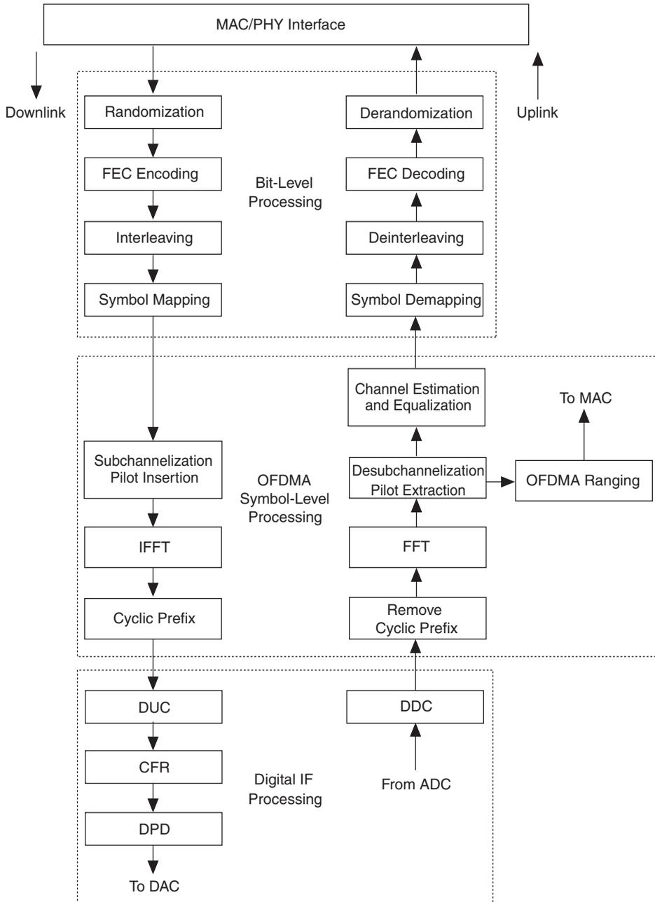
Altera’s WiMAX building blocks include bit level, OFDMA symbol-level, and digital intermediate frequency (IF) processing blocks. For bit-level processing, Altera provides symbol mapping reference designs and support for forward error correction (FEC) using the Reed-Solomon and Viterbi MegaCore® functions.
