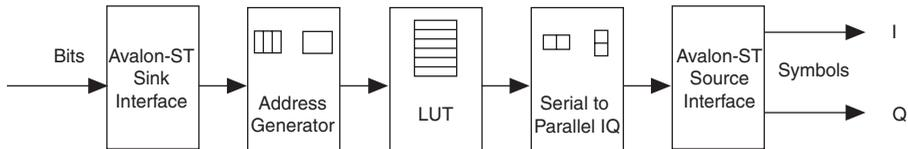
The interleaver presents the input data as a serial bit stream. To generate the symbols, you must group together a number of bits and calculate which constellation point it corresponds to. The address generator groups  $M/2$  bits together to formulate an address where  $M$  is the constellation order. You can use this address to index a lookup table. The lookup table stores the constellation point corresponding to the group of bits.
