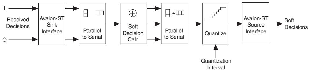
To achieve maximum hardware efficiency, this constellation demapper is fully time division multiplexed. Backpressure is applied to the upstream module so that data is only provided at a maximum rate of one complex sample for every six clock cycles. If data is acquired every six clock cycles, the output bus fully conveys the soft decisions when operating in 64QAM modulation mode. In the 16QAM and QPSK modes, the output bus is not fully used.
