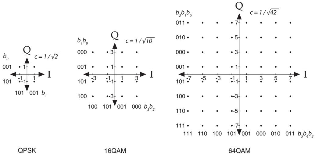
The constellation mapper takes groups of bits and maps them to specific constellation points. A specific magnitude and phase represents a certain combination of bits. The operating mode for each user or subchannel is configured at run time and is determined by assessing the channel quality. The MAC layer adjusts the modulation scheme of each user, to maximize throughput while meeting an acceptable error rate.
