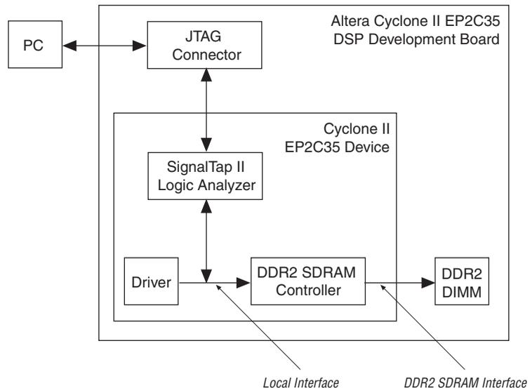
A PC running the Quartus II software downloads the device programming file and monitors the activity on the DDR2 SDRAM interface.
