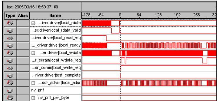
You can zoom in and out with the SignalTap II capture tool to see the writes successfully read back.
