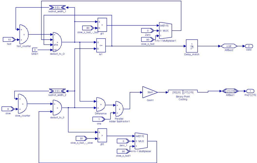
One way to generate the values for μ is to use two counters. Assume the clock ratios can be described as a ratio of  $\text{slow\_clock}/\text{fast\_clock}$ . The lower counter increments by  $\text{slow\_clock}$  until it reaches the value  $\text{slow\_clock} \times \text{fast\_clock}$  and then falls back to 0 again.
