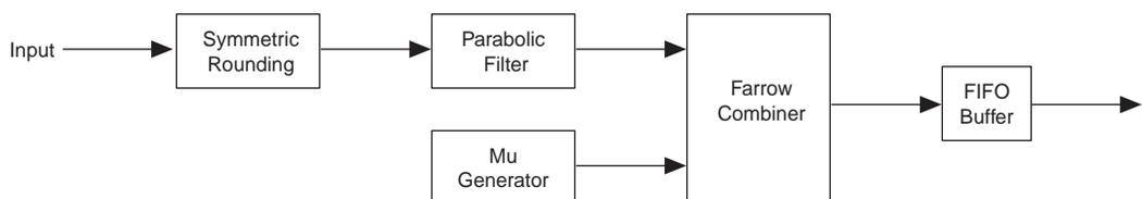
The Farrow-based decimating sample rate converter comprises the following blocks:
