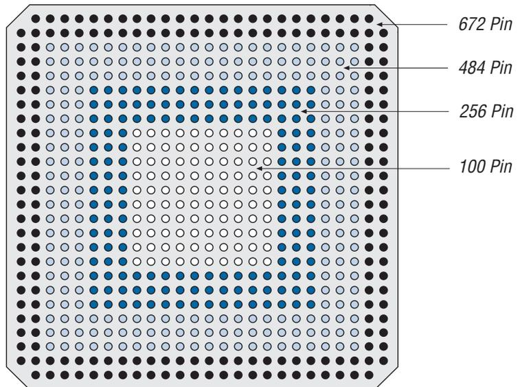
Figure 2 illustrates cross-package migration using 100-pin and 256-pin FineLine BGA packages.
