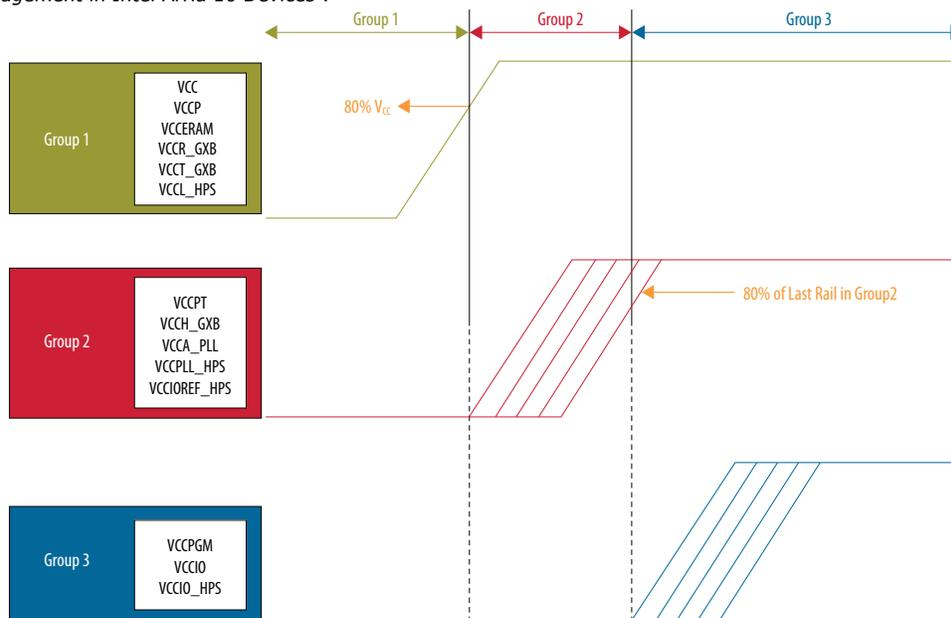
Once you determine your power rail input groupings, use the Early Power Estimator (EPE) spreadsheet to determine the total power required for the input group. The EPE spreadsheet combines the current requirements for each load by summing each FPGA input's current requirement. The result are in in the **Total Current (A)** column in the EPE spreadsheet **Report** tab.
