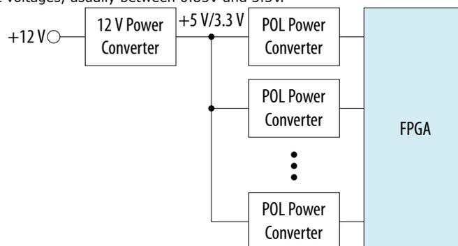
You must determine the input supply voltage and voltage architecture before you select power converters.
