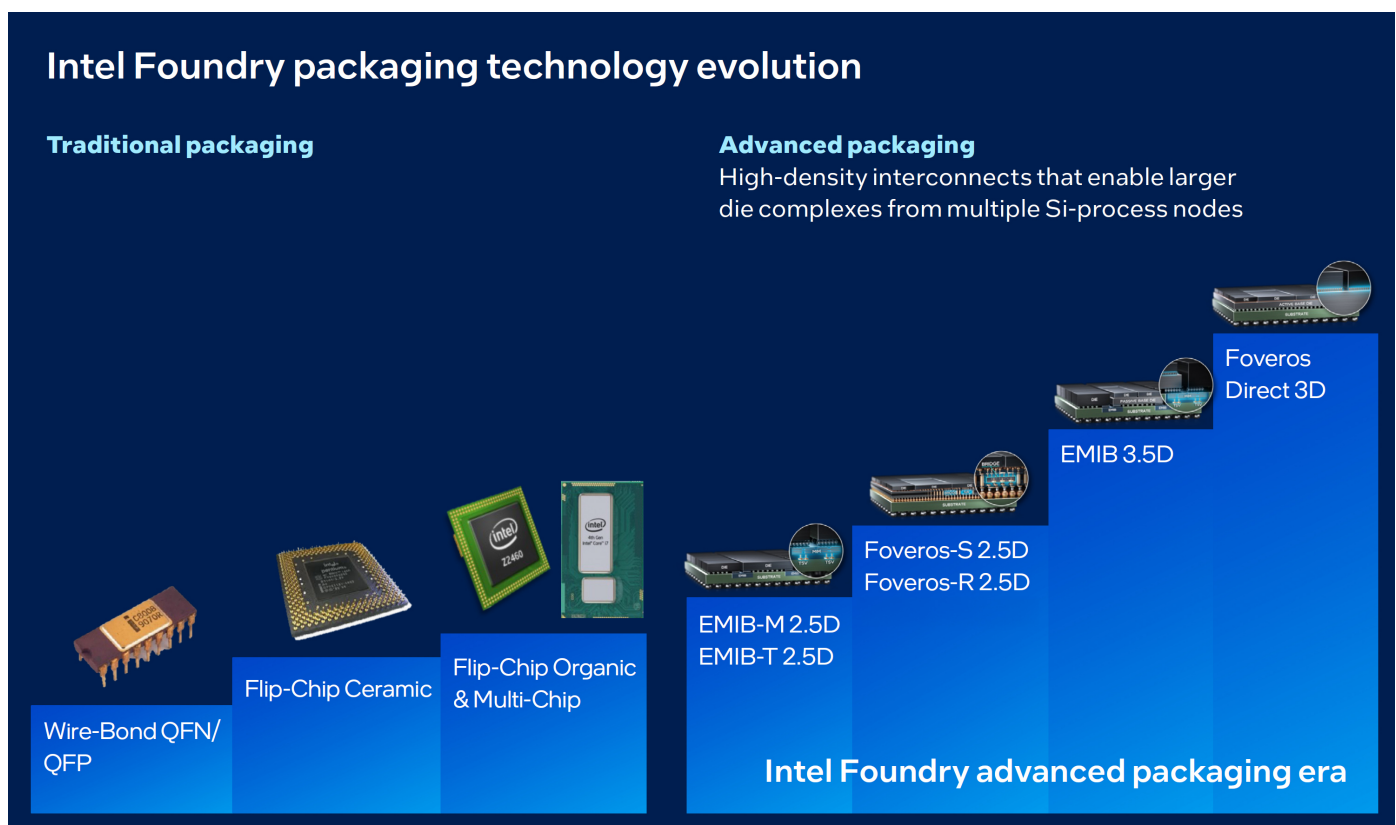
Figure 3. Evolution of Intel packaging technology, from traditional to advanced packaging.
