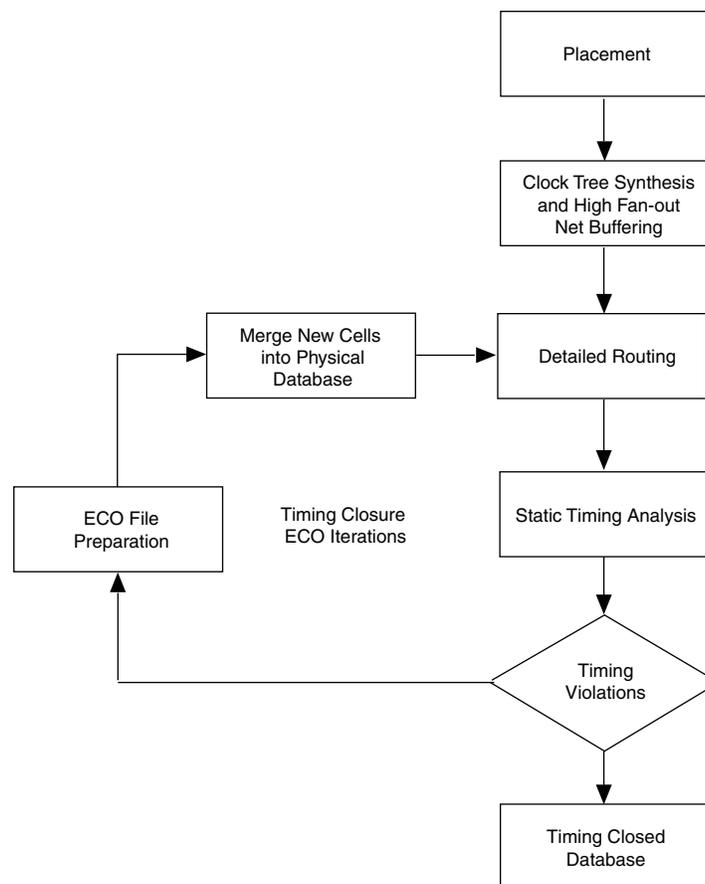
The back-end flow produces the final signoff timing for your HardCopy III device. The Quartus II software produces the timing report for HardCopy III based on global routing and does not factor in the exact physical parasitic of the routed nets. The Quartus II software also does not factor in the crosstalk effect that neighboring nets can have on interconnect capacitance.
