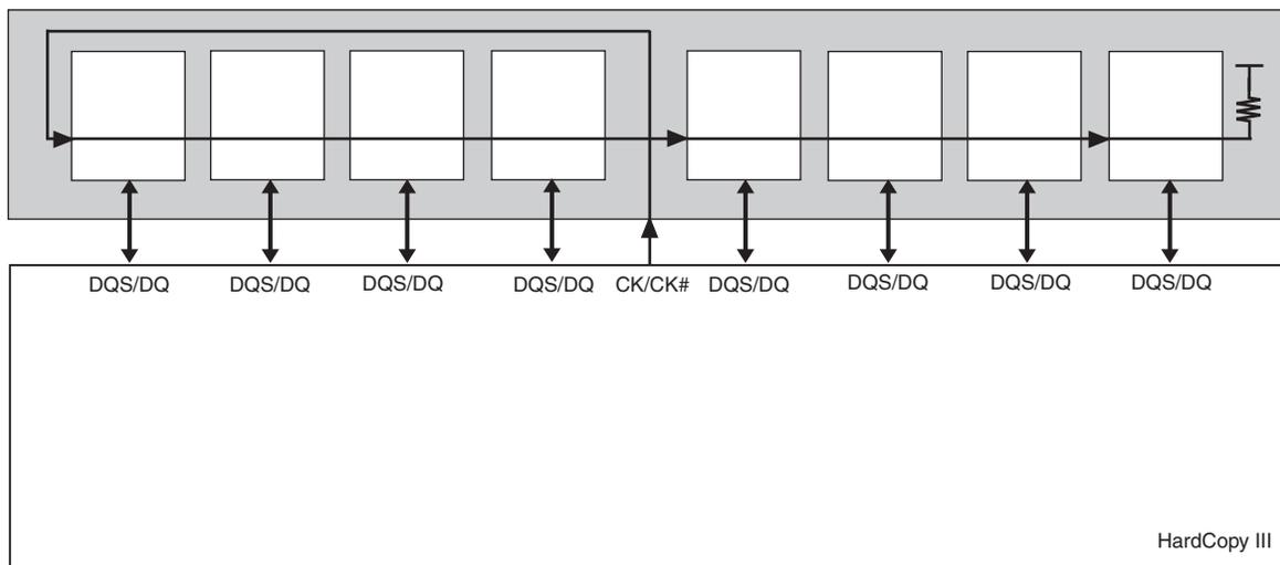
Because the data and read strobe signals are still point-to-point, special consideration must be taken to ensure that the timing relationship between the CK/CK# and DQS signals ( $t_{DQSS}$ ) during a write is met at every device on the modules. Furthermore, read data returning to the HardCopy III ASIC from the memory is also staggered in a similar way. HardCopy III ASICs have leveling circuitry to compensate for the different CK/CK# arrival time at each device in the memory module.
