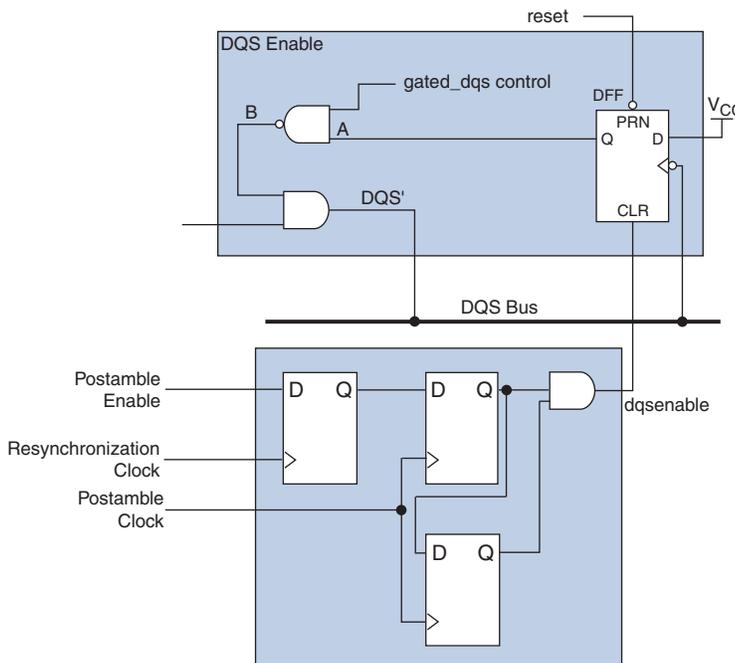
In addition to the dedicated postamble register, HardCopy III devices also have an HDR block inside the postamble enable circuitry. These registers are used if the controller is running at half the frequency of the I/Os.
